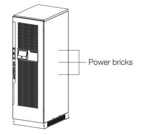
Any potential fault should be isolated inside the affected sub-assemblies, keeping the critical load protected in double conversion mode thanks to the remaining power converters to maximize the Mean Time Between Critical Failure. The UPS will be designed to provide intrinsic double conversion mode redundancy in case of a single power brick is no longer available, to grant a minimum of:
