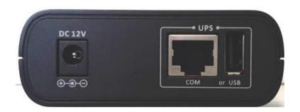
The serial link to UPS is located on the back of the box. The serial cable included in the package has to be connected to 'COM' RJ45 connector and to the UPS RS232 DB9 serial port. The UPS serial COM port used for NET VISION BOX has to be set as following:
