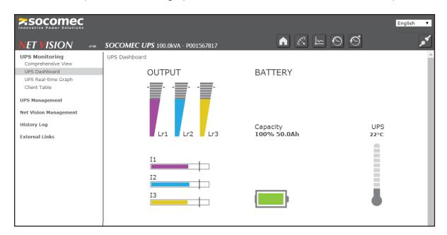
During battery discharging, remaining backup time is displayed
