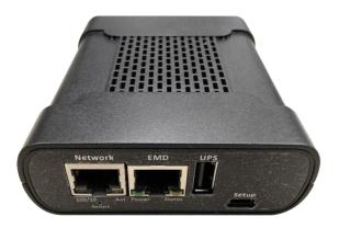
The Network RJ45 connector is used for Ethernet network connection. The EMD RJ45 is used to connect the optional EMD device. Refer to EMD Appendix;
