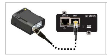
Connect a CAT5 Ethernet cable from NET VISION "EMD" connector to port on the EMD.
