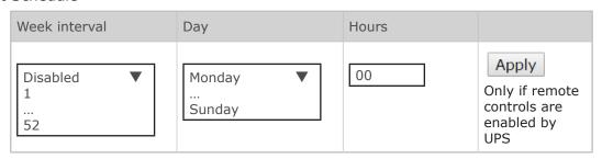
For parallel systems with distributed battery, the battery test schedule can be programmed unit by unit. Each battery test will be started at different time.
