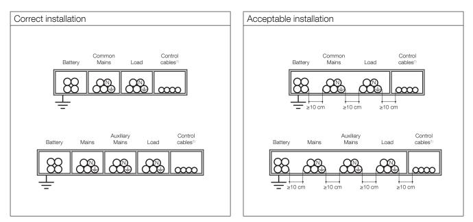
1. Control cables: connections between the cabinets and each unit, alarm signals, remote mimic panel, connection to the BMS (Building Management System), emergency stop, connection to generator.
