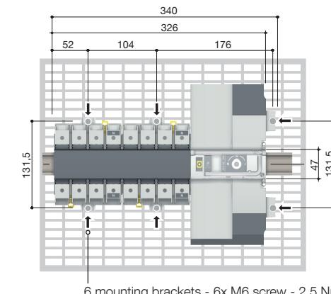
6 mounting brackets - 6x M6 screw - 2,5 Nm
