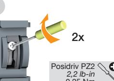
**⚠ Tighten to avoid movement on the DIN rail.**
